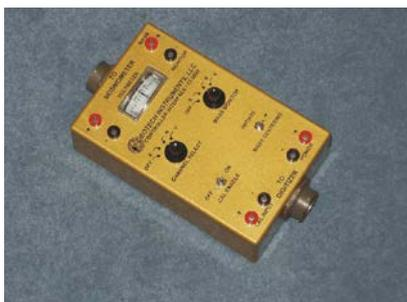
The **CI-2000** Control Interface helps monitoring the mass centering operation. Its manual can be downloaded by pressing [here](#) (0.3MB).
